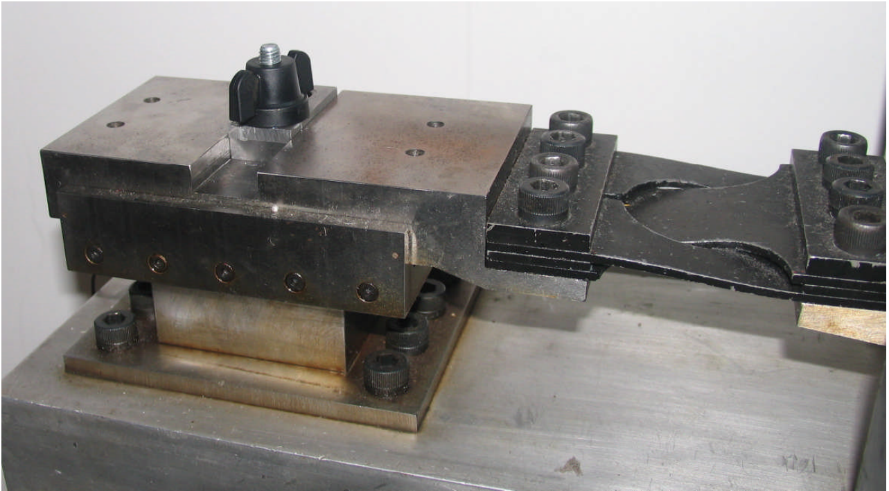
Figure 2 – Under Hole Nut being tested
